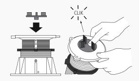
Adjustment from 100 to 175mm by turning the clamp ring
